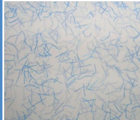
Top: Leonardo with incorporated UV-pigments. Bottom: Distribution of 1% blue viscose fibre in paper
